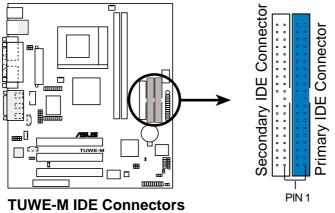
**NOTE:** Orient the red markings (usually zigzag) on the IDE ribbon cable to PIN 1.
